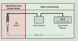
The connection from the moisture sensor to the Zener Barrier is via low loss coaxial cable. The Zener Barrier can also be supplied without the enclosure for direct installation into an existing bus bar system.
